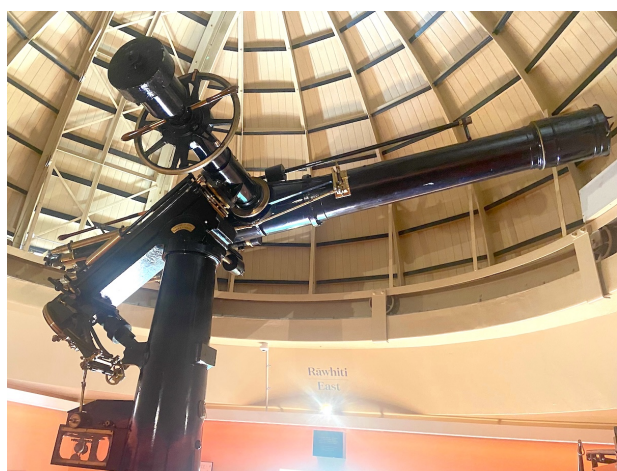
Top: The Mercury Bay Museum Mural. Above: Two views of the Cooke Refractor, a 9 \frac{3}{4} inch refracting telescope by Thomas Cooke of York, at The Carter Observatory, Wellington, New Zealand
