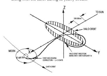
An interesting orbit is followed by the SOHO spacecraft (see drawings), it follows a long oval orbit about the L1 point, 1.5 million km sunward from Earth, about 1/100 the Earth/sun distance, taking 178 days to complete a loop. This position is an excellent one for long term observation of the sun and measuring the solar wind, as it is upwind from Earth by about one hour and just outside the bowshock wave of the Earth's magnetic field interacting with the solar wind.
